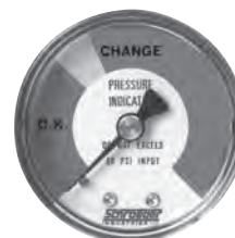
Y2 —Back mounted 1/8" NPT Tri-color Glycerin-filled Gauge (0-60 psi) P/N LFT-134-2 (0-100 psi) P/N LFT-1081 Y2R —Same as Y2 but mounted on opposite side of standard location P/N LFT-134-2 Y2C —Bottom mounted 1/8" NPT Tri-color Gauge (0-60 psi) located in cap P/N LFT-134-3 Y5 —Same as Y2 but located in cap P/N LFT-134-2
